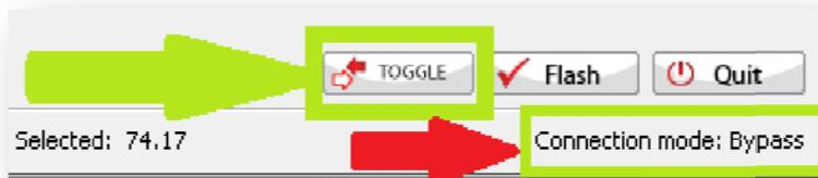
Will switch/toggle the Flash Link Manager connection mode to be use with Bypasses or Remote Starters.
