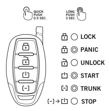
The remote LED flashes BLUE when a button is pressed. The remote LED flashes GREEN when the remote is transmitting the informations. For car command confirmation, see REMOTE START/ALARM DIAGNOSTICS, page 19.
