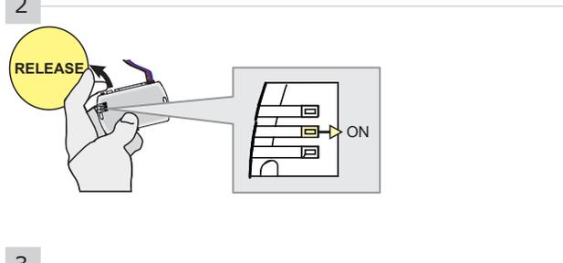
**Release** the programming button when the LED is YELLOW.
