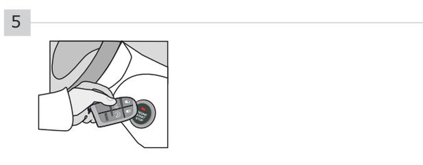
**Place** the OEM remote (no battery) close to the front of START/STOP button exactly as shown.
