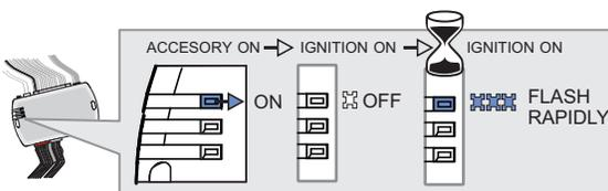
**Press and release** START/STOP button once to turn ON the ignition.
