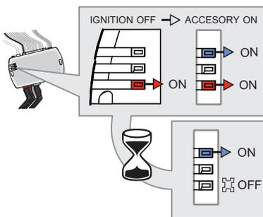
**Press and release** the START/STOP button once to turn ON the ACCESSORY.
