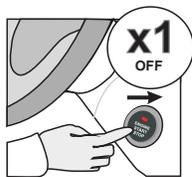
**Press and release** the START/STOP button once to shut off the ignition.
