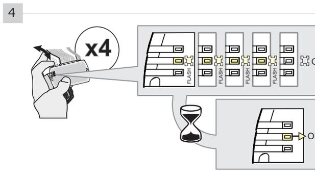
**Press and release** the programming button four times (4x).
