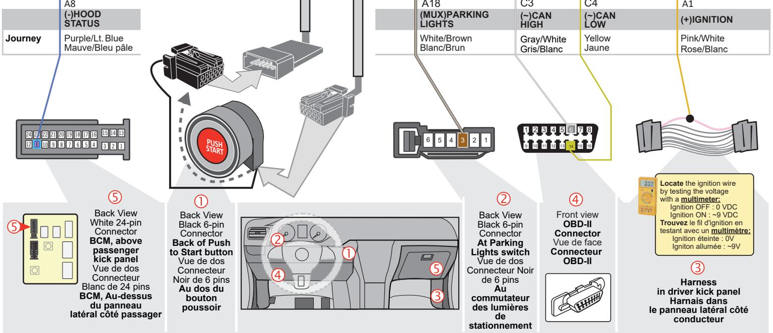
Locate the ignition wire by testing the voltage with a multimeter:
