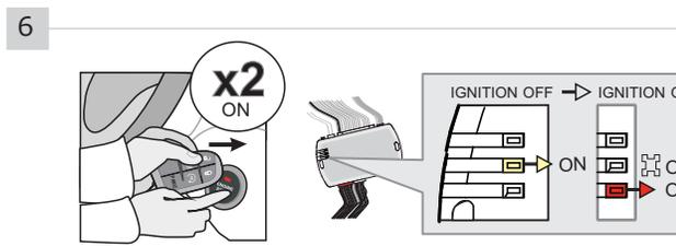
**Press** the Start/Stop button twice to turn ON the ignition.
