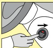
Press the START/STOP button with the key inside the vehicle.
