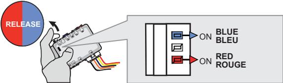
Release the programming button when the Blue & Red LEDs are ON.
