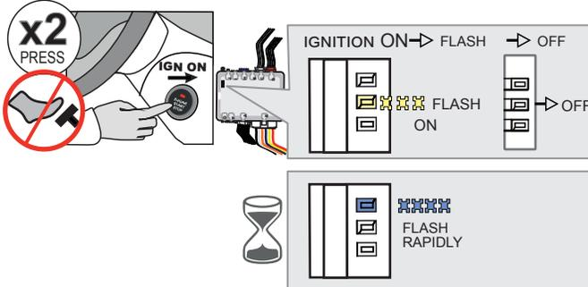
Do not press the brake pedal. Press the START/STOP button twice to turn ON the ignition.
