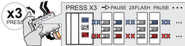
Press and release the programming button three times (3x).
