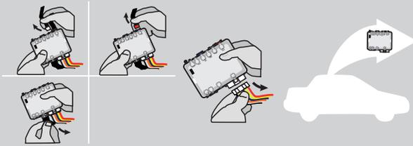
**Disconnect** all connectors and after the 6-Pin (Main-Harness) or the 4-Pin Data-link connector.
