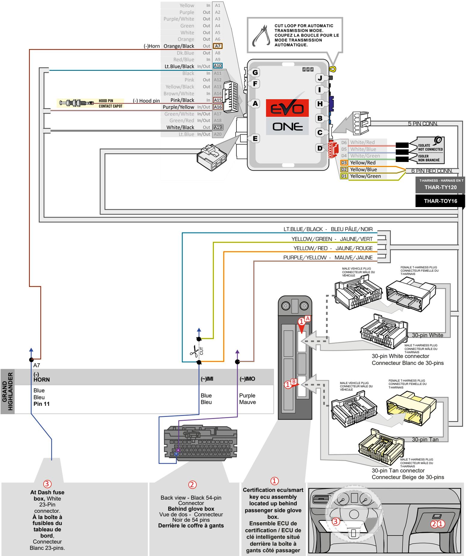
**DCRYPTOR PROGRAMMING PROCEDURE | PROCÉDURE DE PROGRAMMATION AVEC DCRYPTOR**
