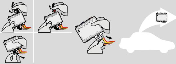
**Disconnect** all connectors and after the 6-Pin (Main-Harness) or the 4-Pin Data-link connector.
