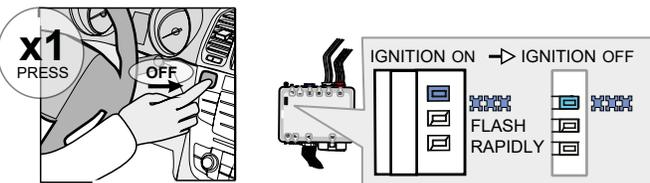
**Press** the Push-to-Start button once to turn the ignition OFF.
