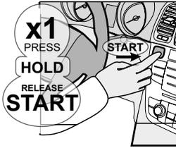
Press the Push-to-Start button until the engine start.
