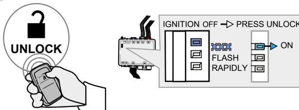
**Press** the Unlock button on the vehicle OEM remote.
