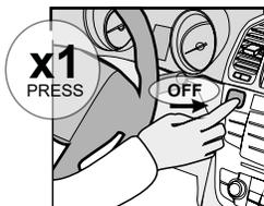
Press the Push-to-Start button once to turn off the engine.
