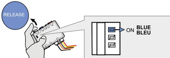
**Release** the programming button when the LED is BLUE.
