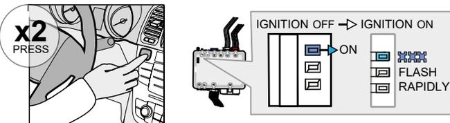
**Press** the Push-to-Start button twice, to turn the ignition ON.
