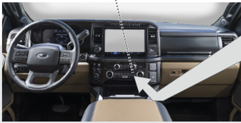
Gateway module, behind audio panel in center dash - 26-pin Black connector.
