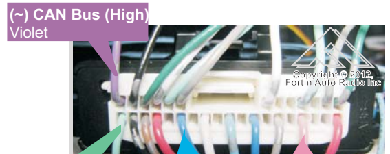
(~) CAN Bus (High) Violet (~) CAN Bus (Low) Lt.Green (-) Push to start Blue (+) Push to start Pink
