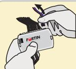
**Verify** all connections. **Disconnect** the 4 Pin connector (Data-Link) and **go back** to step 1.
