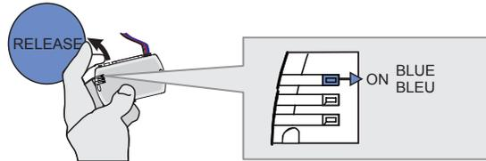
**Release** the programming button when the Blue LED is ON.
