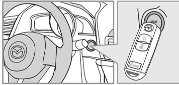
Place the 1st OEM remote close to the front of the START/STOP button exactly as shown.
