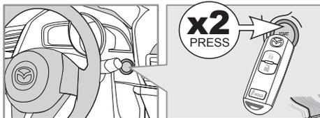
Press the START/STOP button twice to activate the vehicle's Ignition.
