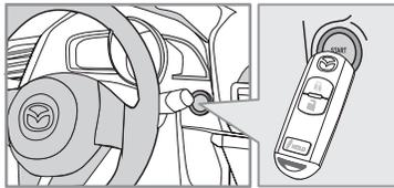
Place the 2nd OEM remote close to the front of the START/STOP button exactly as shown.
