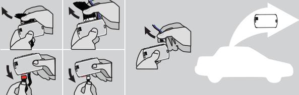
**Disconnect** all the connectors and after the Data-Link (4-pins) connector.
