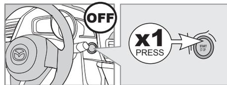
**Press** the START/STOP button once to deactivate the vehicle's Ignition.
