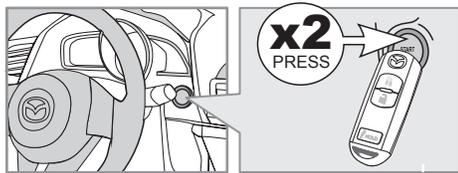
**Press** the START/STOP button twice to activate the vehicle's Ignition.
