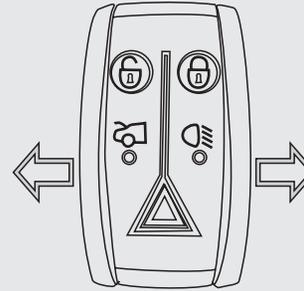
Remove the chrome trim from both sides of the remote. Open the remote.
