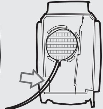
Trim off a small corner inside the remote for the Inset wires and reassemble the remote.
