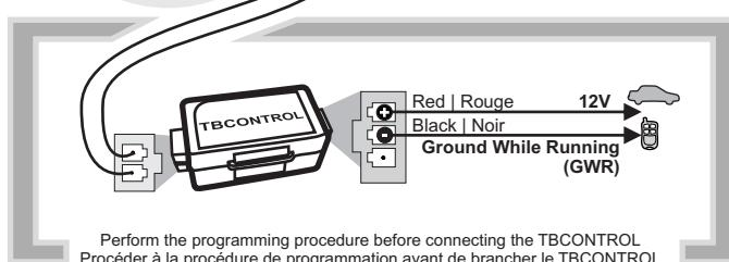
Perform the programming procedure before connecting the TBCONTROL
