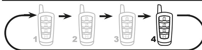
The system can learn up to a maximum of 4 transmitters. Any transmitters can be stored in more than 1 memory slot. When a 5th transmitter is learned the 1st remote is erased (FIFO).
