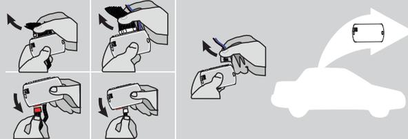
**Disconnect** all the connectors and after the Data-Link (4-pins) connector.
