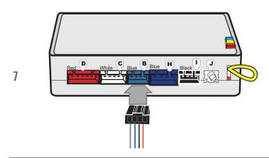
**CONNECT** the REVO in the Blue 4pin connector with clip of the EVO-ONE using a 4pin connector with clip.
