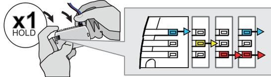
**Press and hold the programming button: Connect the 4-PIN Data-link connector.**
