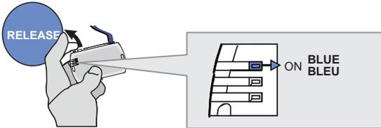
**Release the programming button when the LED is BLUE.**
