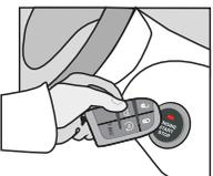
**Place** the OEM remote (no battery) close to the front of START/STOP button as shown.
