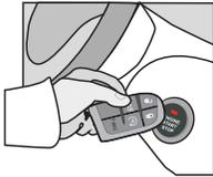
**Place** the OEM remote (no battery) close to the front of START/STOP as shown. Do not move the OEM remote for the following step.
