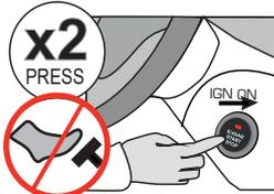
Do not press the brake pedal. Press the START/STOP button twice to turn ON the ignition.
