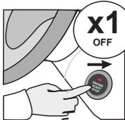
**Press and release** the START/STOP button once to shut off the ignition.
